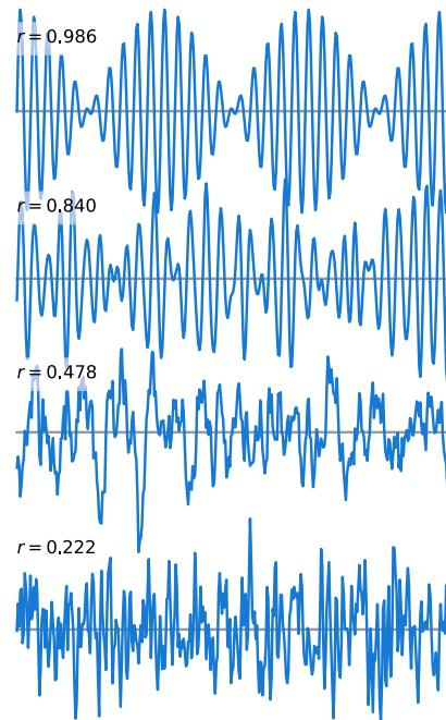
FIG. 1. The crest–trough correlation  $r$  is higher in “groupy,” low-bandwidth sea states. Shown are surface elevations generated from Ochi–Hubble spectra (Ochi and Hubble 1976) with increasing spectral bandwidth (from top to bottom) and the corresponding value of  $r$ .
