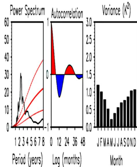
**Figure 7.** Statistical analysis for NINO3 SST anomalies of the years 101–200 for CONT. (left) The variance per frequency band, (middle) the autocorrelation, and (right) the seasonal distribution of the variance. The solid line across the power spectrum marks the variance for an AR(1) process (noise with memory), and the part of the spectrum that is above the uppermost dashed line is significant at the 99% level.
