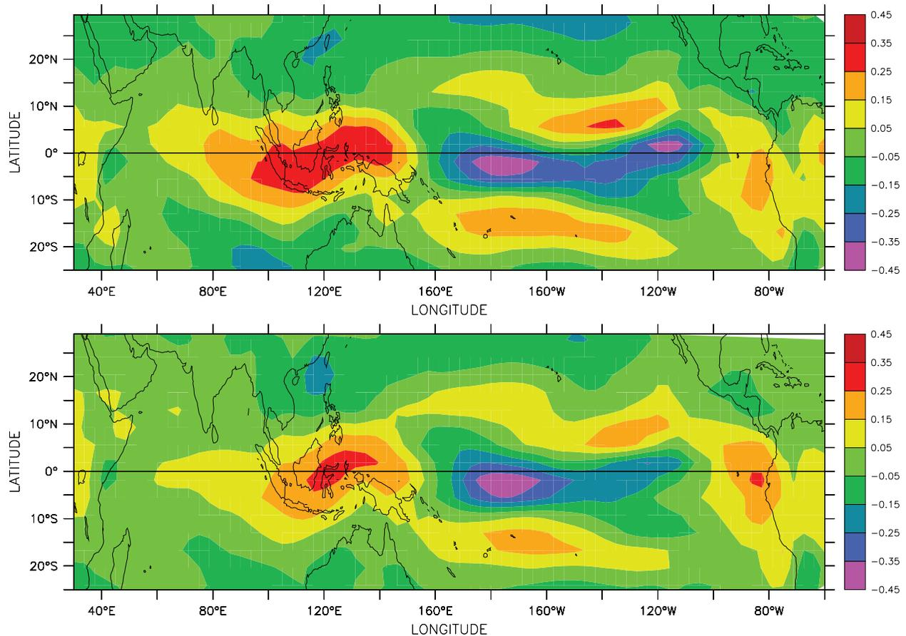
**Figure 11.** Correlation between NINO3 SST anomalies and zonal wind stress anomalies lagging 3 months for (top) CONT and (bottom) PLIO. The weaker correlation in the eastern equatorial Pacific, a key region for the delayed oscillator [Neale *et al.*, 2008], indicates a weaker coupling between equatorial SST and off-equatorial wind stress.
